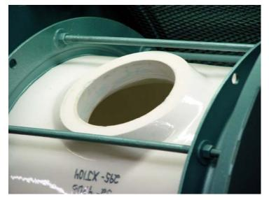
Loading and unloading is accomplished through a large port located on the peripheral surface of the mill cylinder. A solid ceramic cover completes the surface continuity when the mill is rotating, while screen or grid-like discharge covers are available in different forms for wet or dry discharging. These discharge covers retain the grinding media while permitting the material to be removed.
