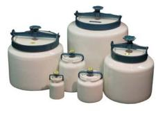
Mill jar sizes range from ½ pint to about 6 gallons total capacity. Jars 6 gallons and larger are quite unwieldy and often require special handling equipment. Mill jars most commonly used are made of alumina fortified ceramic material, formed with a wide opening neck for easy loading and unloading. They are also available in high alumina material, unlined stainless steel, carbon steel and rubber or polyurethane lined steel.
