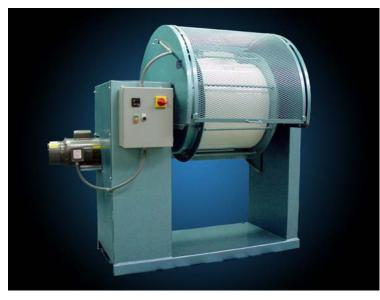
**Basically, a mill consists** of a horizontal vessel whose length exceeds its diameter. The vessel is fitted with shafts and rotated about its longitudinal axis. There are, however, some exceptions where the diameter exceeds the length. By increasing the diameter of the mill, and reducing the length, the efficiency of operation increases. This is caused by the greater height of fall and impact energy imparted to the grinding media because of the
