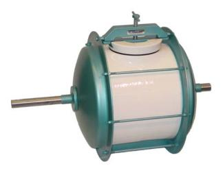
The second design (shown at the right) is used on larger mill sizes (87, 117, and 210 gallon). Cylinder liners are of the same high alumina ceramics, made with three cylinder shaped ceramic pieces and two ceramic end caps. The cylinders are fired together to form one piece and the end caps are ground and lapped to form a liquid tight seal providing a very low contaminate milling environment. The finished cylinder is then reinforced and completely protected by a flanged steel casing.
